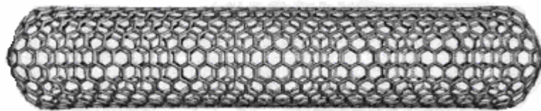
Figure 1.5 Molecular Model of a Carbon Nanotube Capped by Six Pentagons in Each End, from Terrones, 2003.
